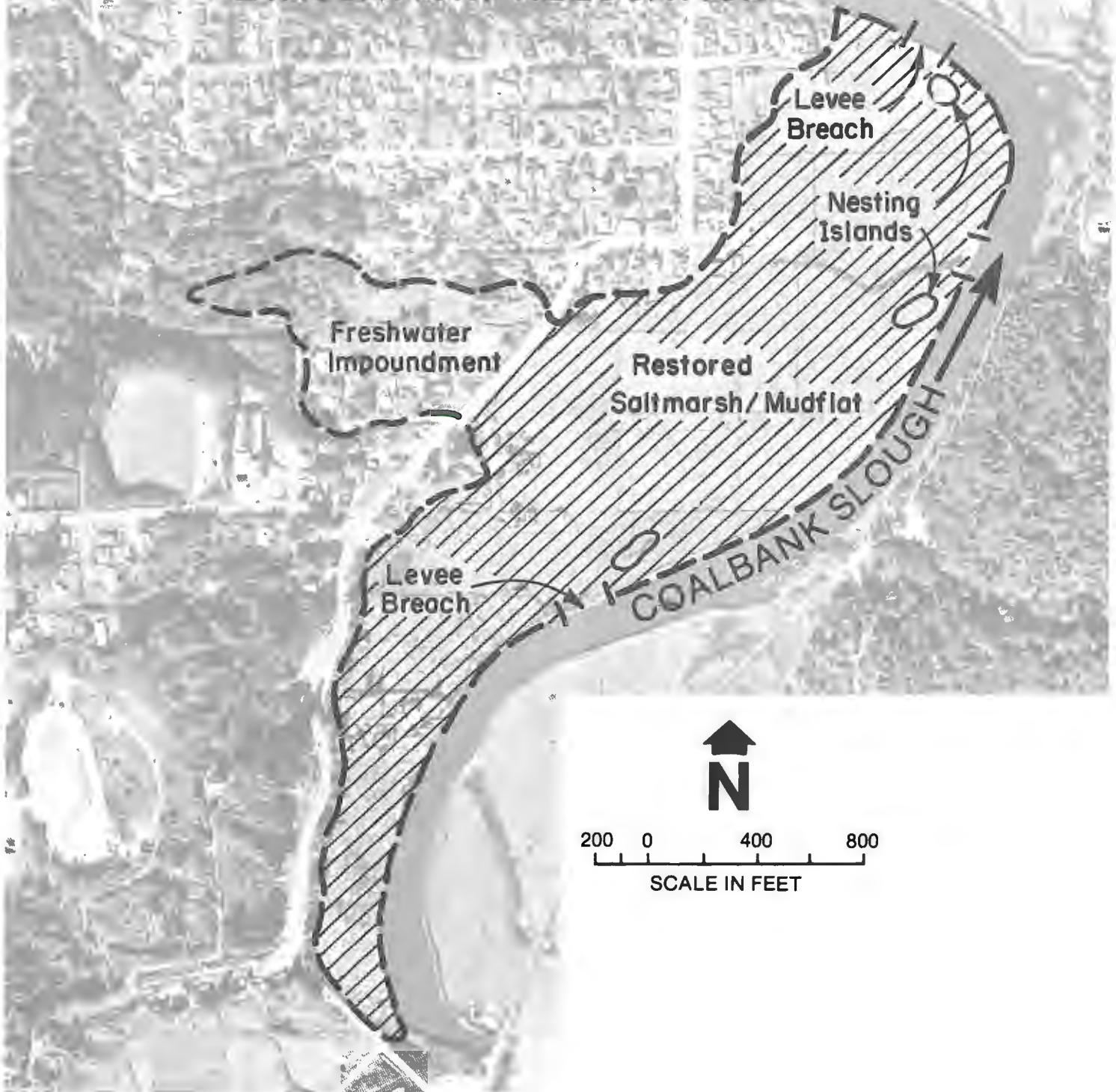
Figure 8. Permanent Floodplain Evacuation - Alternative 4.
